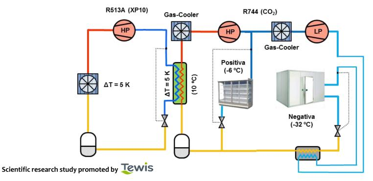
Cascade system + basic CO, booster + Parallel compressor (Subcritical)
